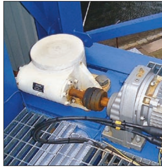
(Above) Isleburn Mackay & Macleod used the Internet to download engineering drawings of the Nook 50-ton ball jacks they needed to complete the Aberdeen Ferry Bridge.
