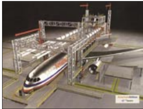
(Above) Uni-Dock, a sophisticated maintenance docking system for Boeing 777 and 767 class aircraft, moves heavy loads vertically and horizontally to allow the plane to enter and exit the docking system. Nook ball screws were selected because they were the most efficient mechanisms for moving heavy loads, required the least amount of horsepower to operate, provided reliable safety features, and were cost-effective.
