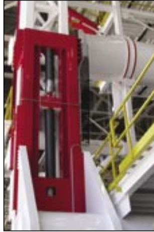
(Above) Four Nook ball screws with a built-in safety nut feature, such as the one shown here, lift the main bridge of the Uni-Dock, a load of 100,000 pounds per screw.
